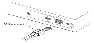
4. As a connection is made, check the Activity LED on the switch's front panel for the corresponding module to be sure that the connection is valid.
